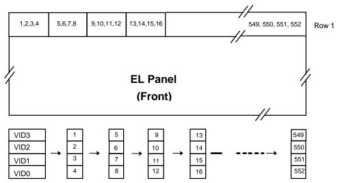
Figure 4. Pixel Location vs. Sequence of Data
